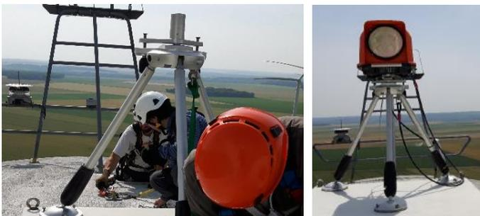
As well as installing the LIDAR equipment, Laborelec takes care of all the other aspects of the campaign, from the preparation of safety documentation to remote monitoring and data analysis.
