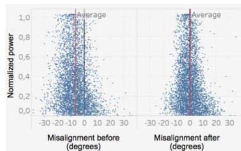
The LIDAR measures the precise magnitude of the static yaw misalignment. Then, after the corrections are carried out, the LIDAR confirms the effectiveness of the operation. The resulting increase in annual energy production can be as much as 5 %.
