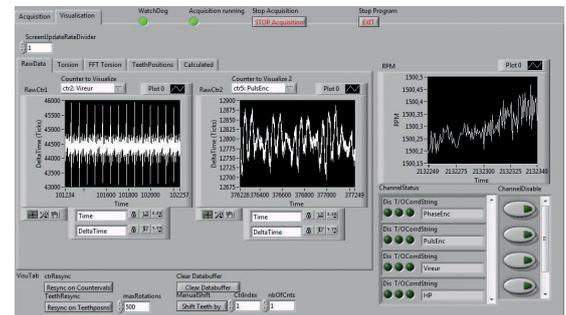
Alarm thresholds set too high will lead to undetected excessive torsional vibration and severe damage. However, excessively low thresholds can generate a large number of unwanted alarms. The model behind TORSO makes it possible to calculate precise thresholds, and determine a safe middle course.
