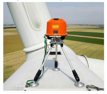
With LIDAR, wind speed and orientation are measured ahead of the turbine, by sensing so-called "free wind". This is much more accurate than data from anemometers positioned to the rear of the nacelle, which measure the more turbulent air behind the blades.
