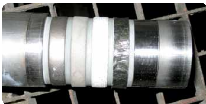
Laborelec invested in an online corrosion monitoring system to determine the corrosion rate of boiler materials when co-firing various biomass and coal blends.
