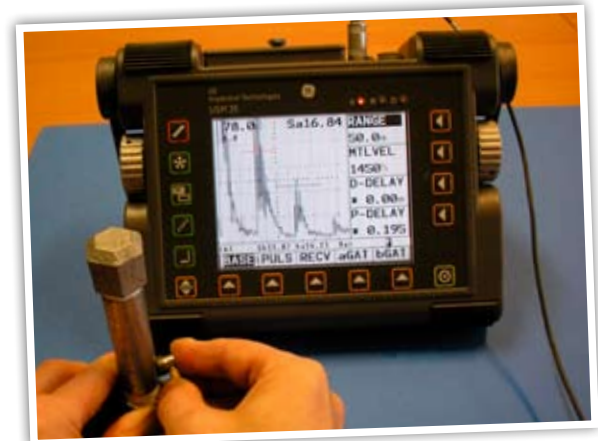
The ultrasonic testing device can determine the level of any substance in a tube, without disturbing operations.
