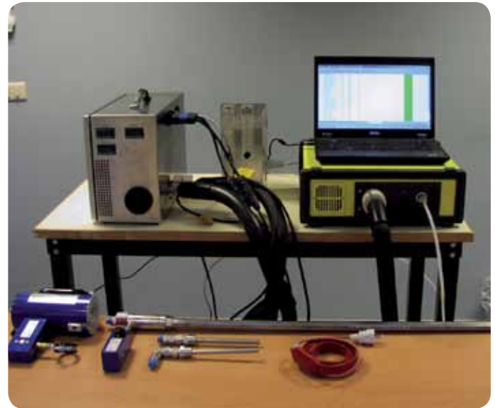
The FTIR monitoring tool enables Laborelec to measure organic substances in the flue gas emissions of PCCC plants.
