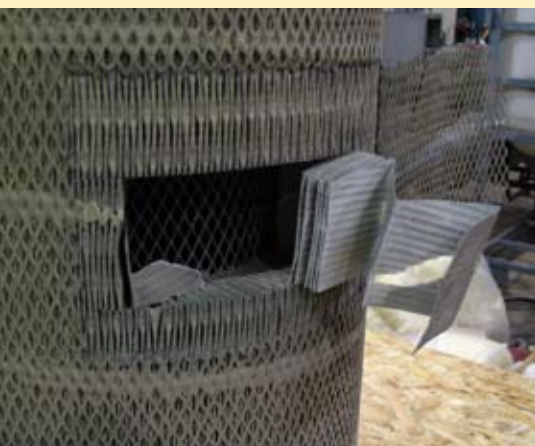
The visual analysis of the Oman filter clearly showed a complete penetration of the filter material.
