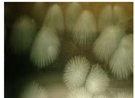
By accelerating the growth of water trees in laboratories, their evolution can be better understood.
