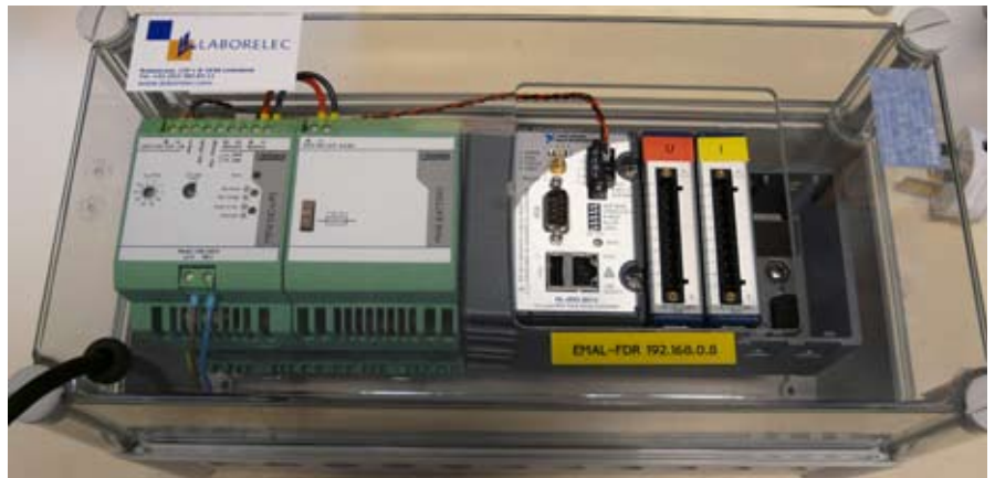
Laborelec developed a monitoring device that records the sine waves of current and voltages before and after a variation.
