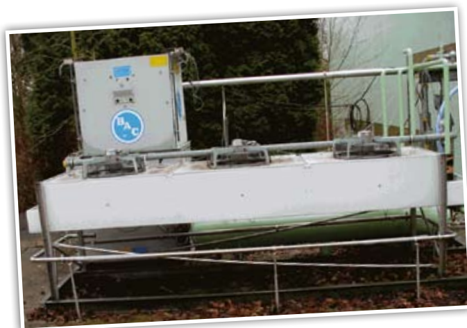
By developing a 3m x 1m model of an air-cooled condenser, our experts monitored scaling.
