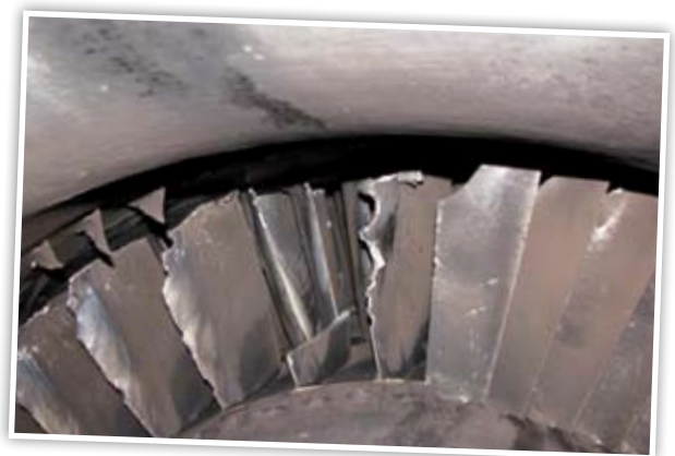
The root cause analysis of the broken compressor blade was executed by the OEM in close collaboration with Laborelec.
