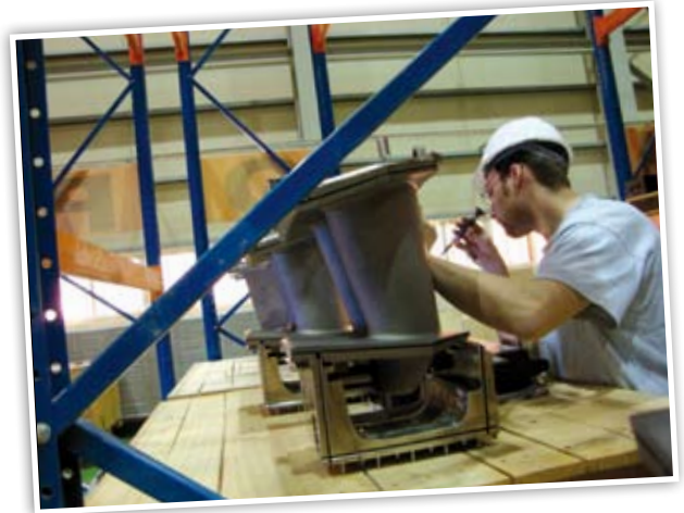
Laborelec's in-house checklist ensures efficient and comprehensive inspection of gas turbine components.
