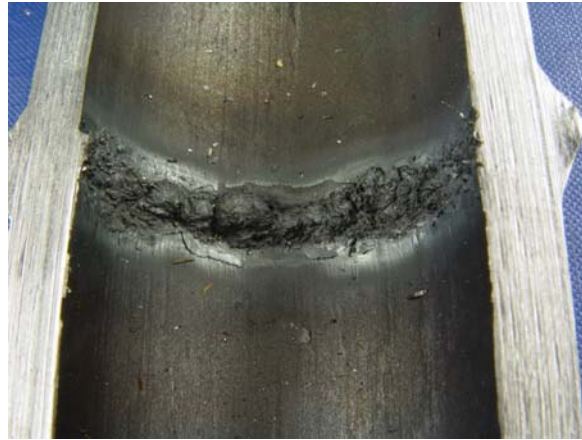
Figure 3: Oxidation of the root bead (dia. 50.8*7mm)
